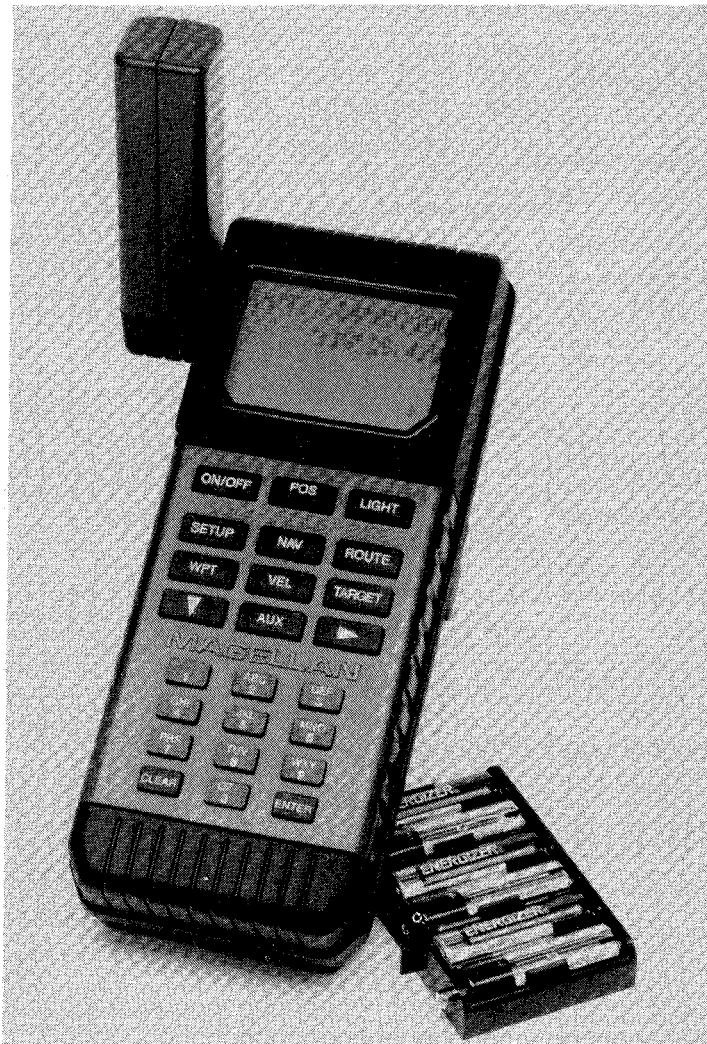
Fig. 8. Commercial one-channel hand-held GPS receiver and position and course computer - position accuracy about 25 yd (courtesy Magellan Systems Corporation).
